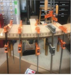
Construction of a solid maple coupler rail for new combination pistons above the pedals.
